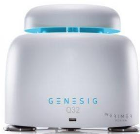
Rapid heating and cooling makes the genesig q32 one of the fastest qPCR instruments on the market today. Assembled from just a few building blocks, this robust qPCR instrument allows analysis of up to 32 samples in both tube or strip format. The powerful genesig q32 software is easily installed from a USB flash drive onto any PC or Mac. The genesig q32 used together with the dedicated genesig kits provide:
